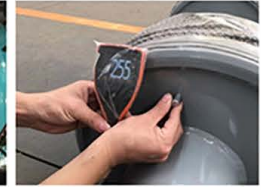
Carrying Out Paint Film Thickness Inspection (DFT)
