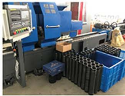
HDPE Rollers - Extruding and Cutting
