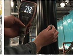
Carrying Out Paint Film Thickness Inspection (DFT)
