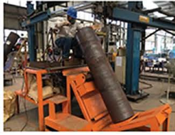
Welding by SAW
