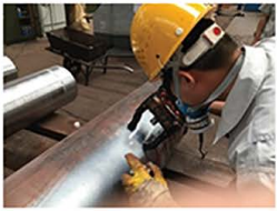
Magnetic Particle Inspection
