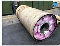
Dye Penetrant Inspection on Stainless Steel Pulley
